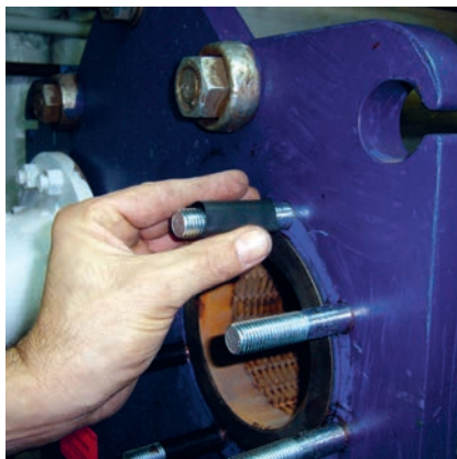
SHUFFLE THE SHRINKING HOSE ABOUT THE BOLT
